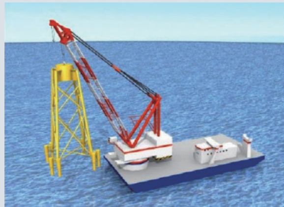
②Jacket Installation (image)
