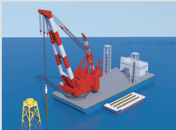
①Pile Installation (image)
